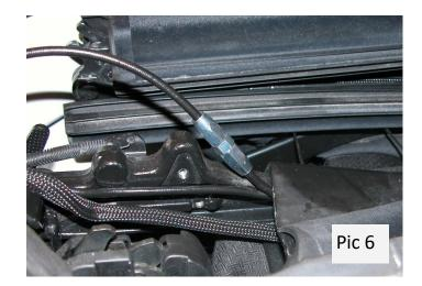
Pic 6 shows the new hose section reattached with the coupler.
