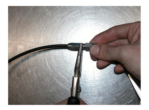
**Step 5**: To prevent cross threading, thread the crimping nut onto the coupler by hand until resistance is felt. The nut should be 1/8" away from the center hex of the coupler
