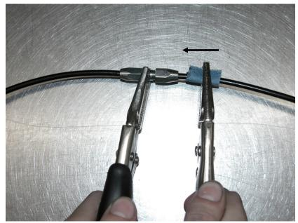
**Step 1:** Clamp coupler with locking pliers around the center hex of the coupler body .
