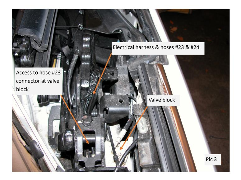
Pic 3 shows the hose and harness cover removed. Also shown are the valve block and rectangular opening to access the hose #23 connector at the valve block. Utilizing suitable tools such as long needle nosed plyers, hemostats, and a long thin flat screwdriver, it is possible to remove and replace #23 connector from the valve block without lifting the top frame. The top frame will have to be lifted out of the way to gain access to hose connector #24 if that hose is damaged.
