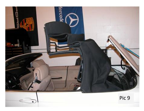
**Step 7:** Move the top so that the main bow is in a vertical position as shown in Pic 9.
