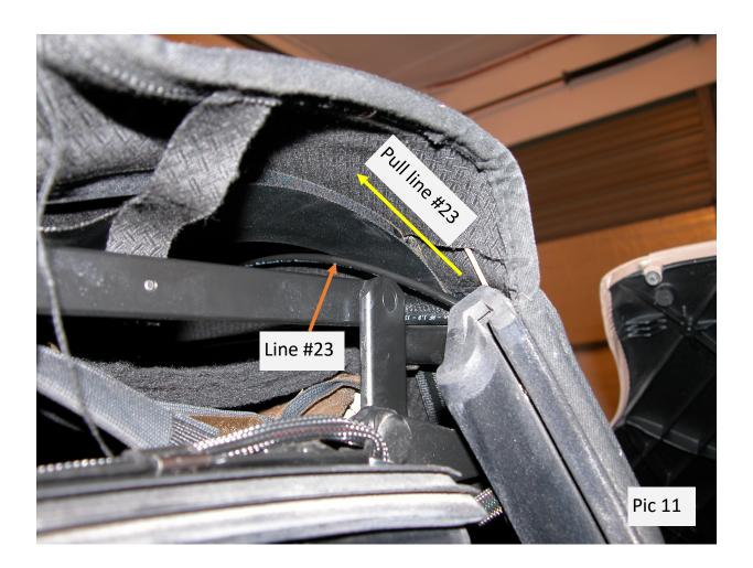
**Step 9**: Begin at the top left corner of the main bow and pull hose #23 as shown in Pic 11. The extra slack will build up at the top of the bow and the hose may become detached from the plastic clips located along the top of the bow frame. The hose can be clipped back into postition after the next step. To identify which hose to pull, simply choose one and pull on it. You've chosen the correct hose when the coupler joint moves.
