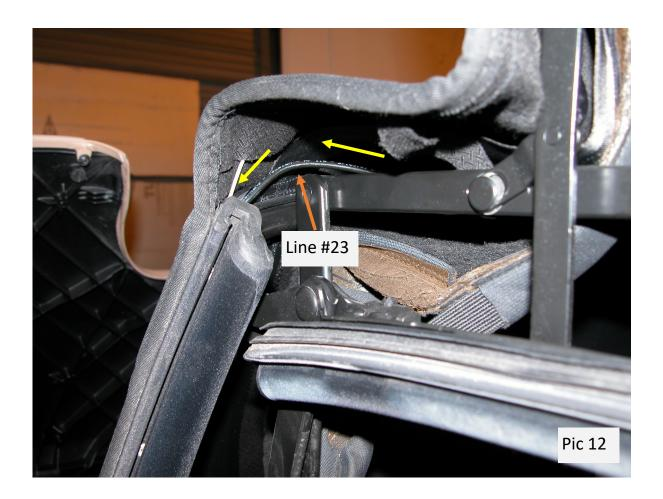
**Step 10:** At the top right corner of the bow, Pic 12, pull the hose to take up the slack and insert the hose back into the plastic clips if they became detached.
