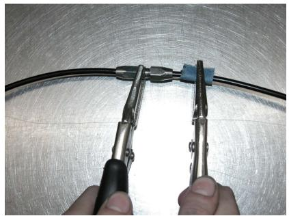
**Step 2:** Clamp coupler with locking pliers around the center hex of the coupler body.
