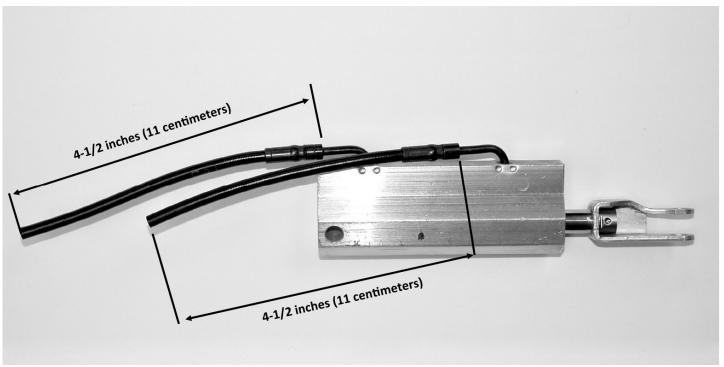
Cylinder orientation for Ferrari 360 & 430 Spider as seen with the front section of the top flipped back, P/N 6645700.
