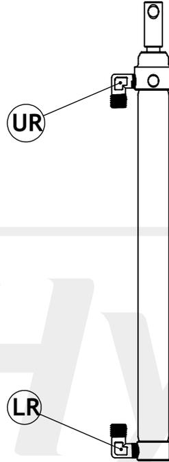
UL & UR pump connections are interchangeable
