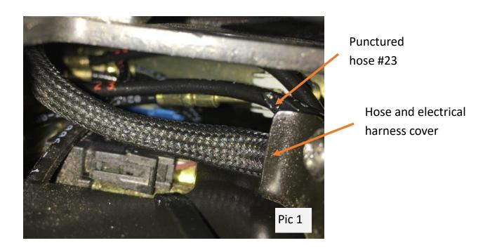
Pic 1 shows a punctured hose #23 and the front edge of the hose and electrical harness cover.
