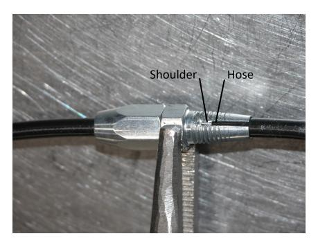
**Step 3:** Unscrew the crimping nut and slide away from the coupler .
